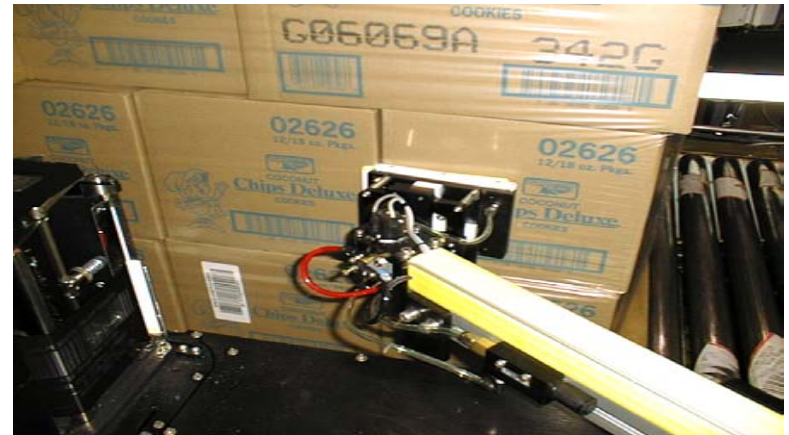
The Apax print/apply labeling systems used in the Pallet Trak system feature an adjustable swing arm that provides front/side or side/rear pallet labels. Some suppliers make the mistake of recommending corner-wrap labeling equipment for pallet identification applications. While suitable for carton applications, our experience has been that pallet loads do not present the standard, consistent corner position necessary for corner-wrap labeling systems to function properly. As a result, only a portion of the long label ends up on the proper area of the pallet. Apax's swing arm design ensures that one to four individual labels are properly applied. Because it is adjustable, labels can be applied to left or right corners or in the center of the pallet load.
