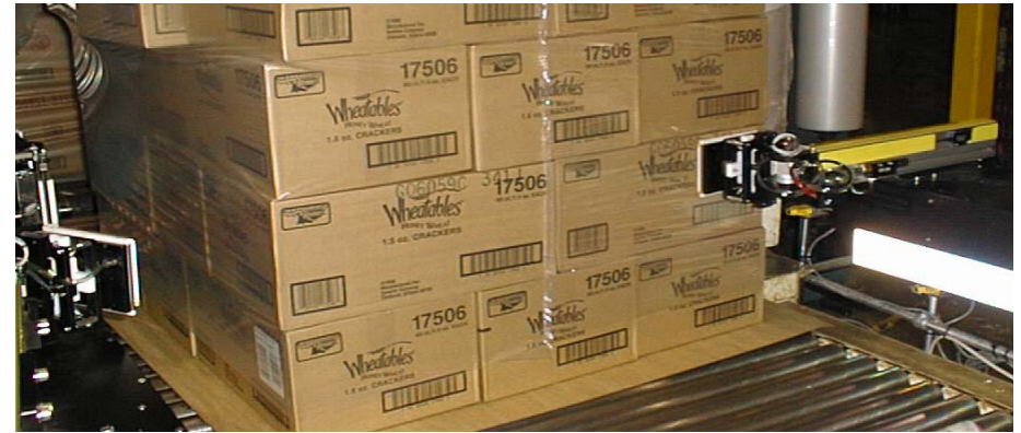
Apax printer/applicator applying a UCC128 label to the front panel of a pallet. This system can print and apply unique labels to pallets at a rate of 20 labels per minute.
